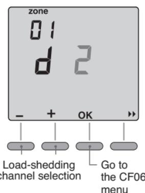
Press and release button . The green LED stops flashing. Receiver A is associated with zone 1 and load shedding channel d=2.
