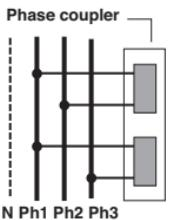
In three-phase installations, you must use a phase coupler to transmit on the 3 phases simultaneously (ref. 6051046)
