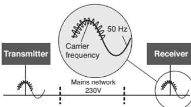
The DELTA DORE X2D protocol conforms to the NF-EN50065-1 standard which allows several PLC systems that comply with the standard to coexist in one installation.
